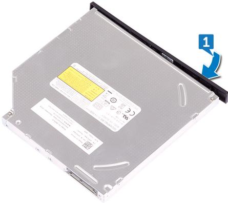
2. Place the slim optical-drive assembly on the slim optical-drive bracket and snap the slim optical-drive assembly in place.
