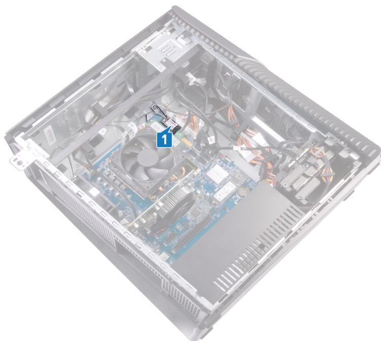
2. Remove the screw (M2x3.5) that secures the wireless card to the system board.
