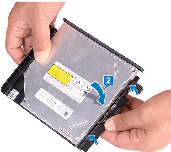
3. Slide the slim optical-drive assembly into the slim optical-drive bay through the front of the computer.
