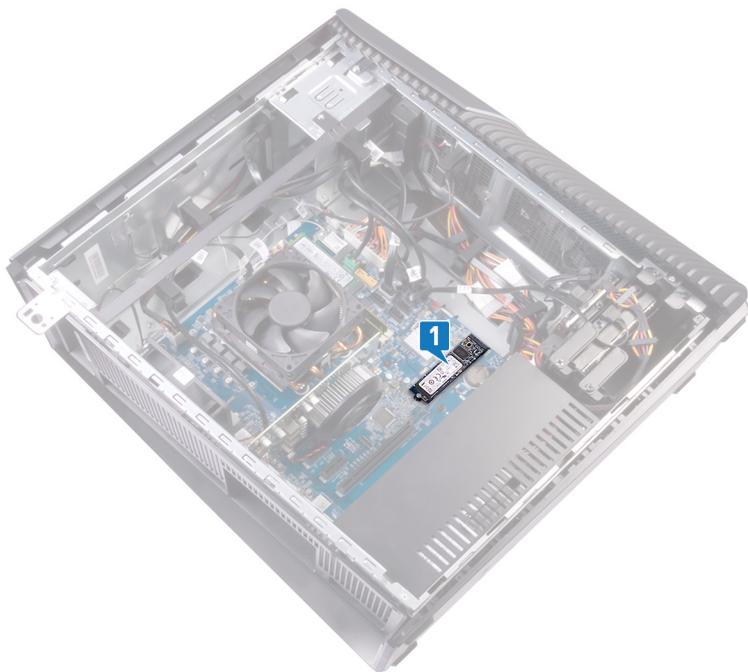
2. Remove the screw (M2x3.5) that secures the solid-state drive to the system board.
