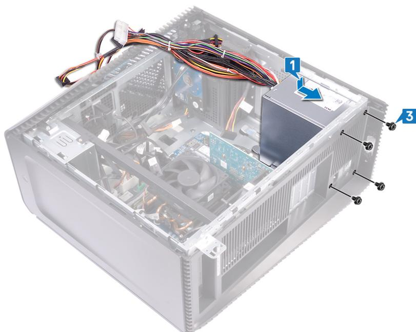
4. Route the power-supply unit cables through the routing guides on the chassis.
