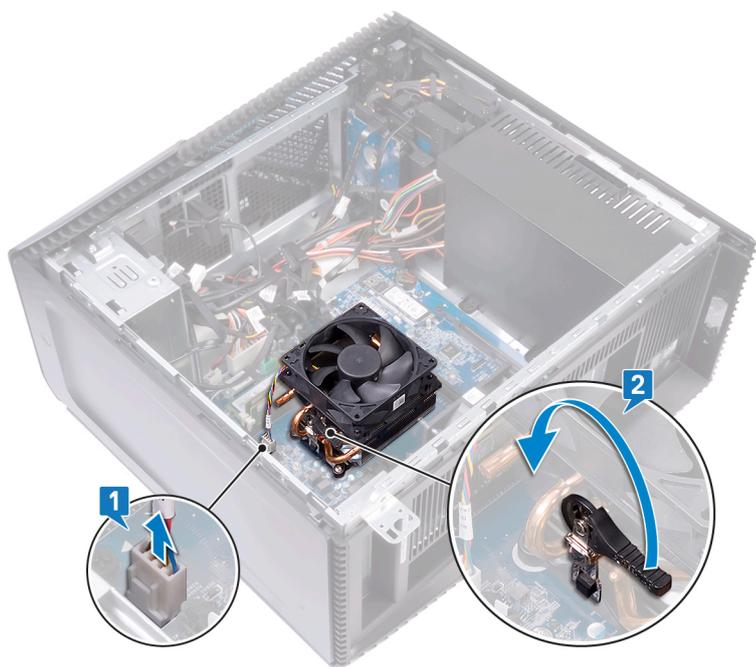
3. Press the lever and release it from the securing tabs on both sides of the processor.
