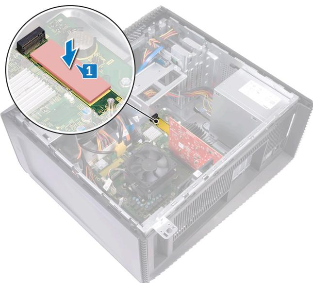
2. Align the notch on the solid-state drive with the tab on the solid-state drive slot.
