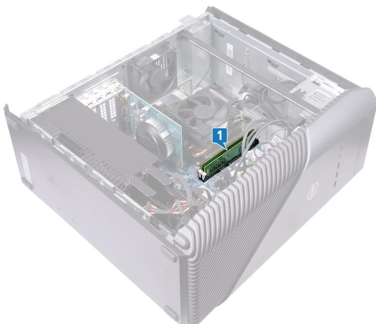
2. Using your fingertips, spread apart the securing clip at each end of the memory-module slot until the memory module pops up.
