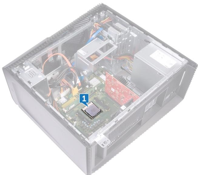
2. Press the release lever down and then push it away from the processor to release it from the tab.
