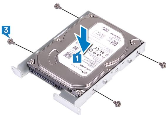
4. Slide the hard-drive assembly into the slot on the side-chassis.
