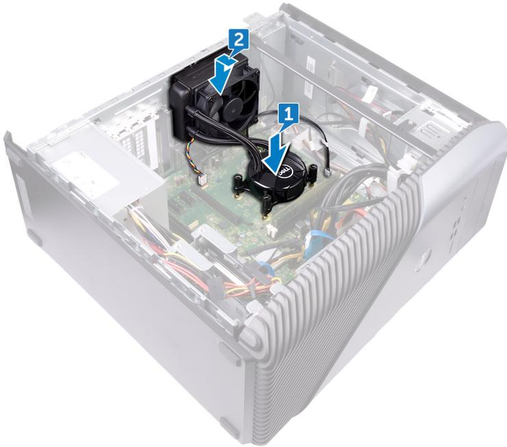
3. In sequential order (as indicated on the processor-cooling assembly), tighten the captive screws that secure the processor-cooling assembly to the system board.
