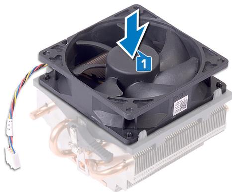
2. Align the processor fan and heat-sink assembly to the slot on the processor.
