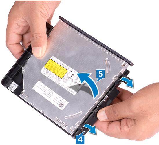
6. Remove the slim optical-drive bezel from the optical drive.
